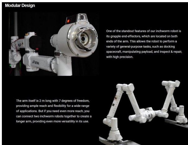
Figure 4: GITAI Inchworm Robotic Arm Capable of Hosting Disassembly End-Affector [6]
